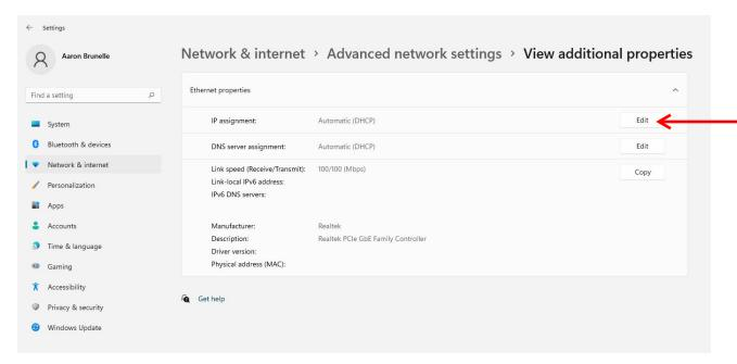
6. Click the drop-down and select "Manual". Then switch IPv4 to "On". Then, for the IP address take the IP address on the controller and increment/decriment it by 1 (i.e. if the controller IP address is 10.0.100.112, use 10.0.100.113 or 10.0.100.111). For the Subnet mask match the Subnet mask on the controller. Leave all other settings alone. Then press the Save button to exit. Then click on "Advanced network settings".
