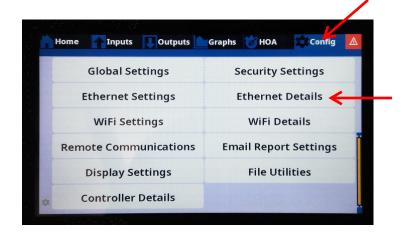
2. In the Ethernet Details sub-menu, swipe up and down through the options until you find the Controller IP and the Netmask. Make a note of these as they will be used in the direct ethernet connection proceedure. The default IP address is 10.0.100.101 and the default subnet mask is 255.255.254.0.
