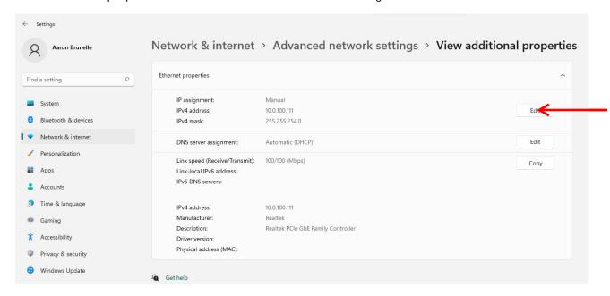
10. Click the drop-down and switch back to "Automatic (DHCP)". Then press the Save button to exit. Then click on "Advanced network settings".
